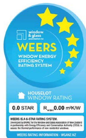
Figure 4. A WEERS label shows the thermal performance of windows.
