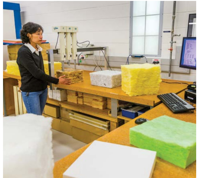
BRANZ Technician Sheng-Huei Huang tests the thermal performance of insulation, the minimum requirements for which are increasing significantly for roofs.
