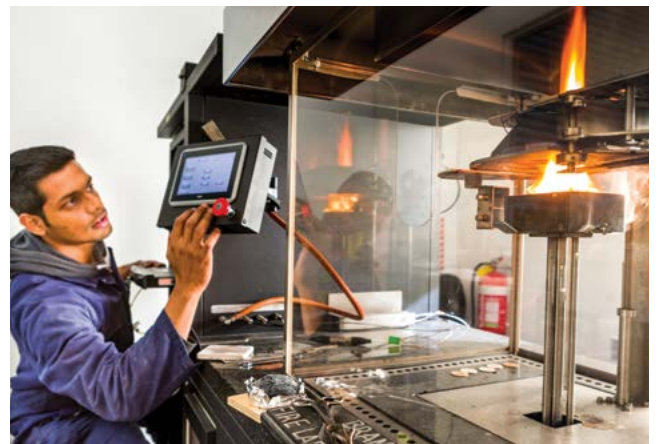
BRANZ Senior Fire Technician Aman Kumar tests an engineered wood product to help understand its expected performance in a real fire.
